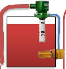
Screw in the straight 1/4" x #6 JIC fitting to the side of the FCV. Next push the swivel fitting onto the blue 3/8" pilot hose then connect it to the JIC fitting in the FCV and run it down to the FIV. Now connect the red breather hose to the spout on the FCV then secure it with the hose clamp and let it hang down the fuel tank where it will be out of the way. At ground level connect the blue pilot hose to the #6 fitting in the FIV.
